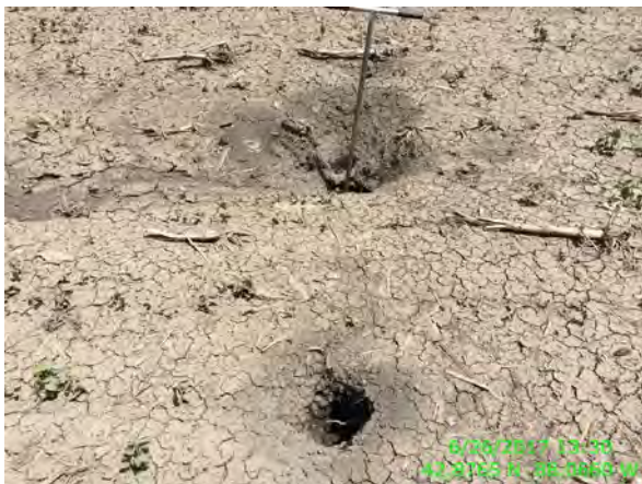
Photo #53 Tile blowouts in a line along east-west main in farmed wetland W-3, view east.
