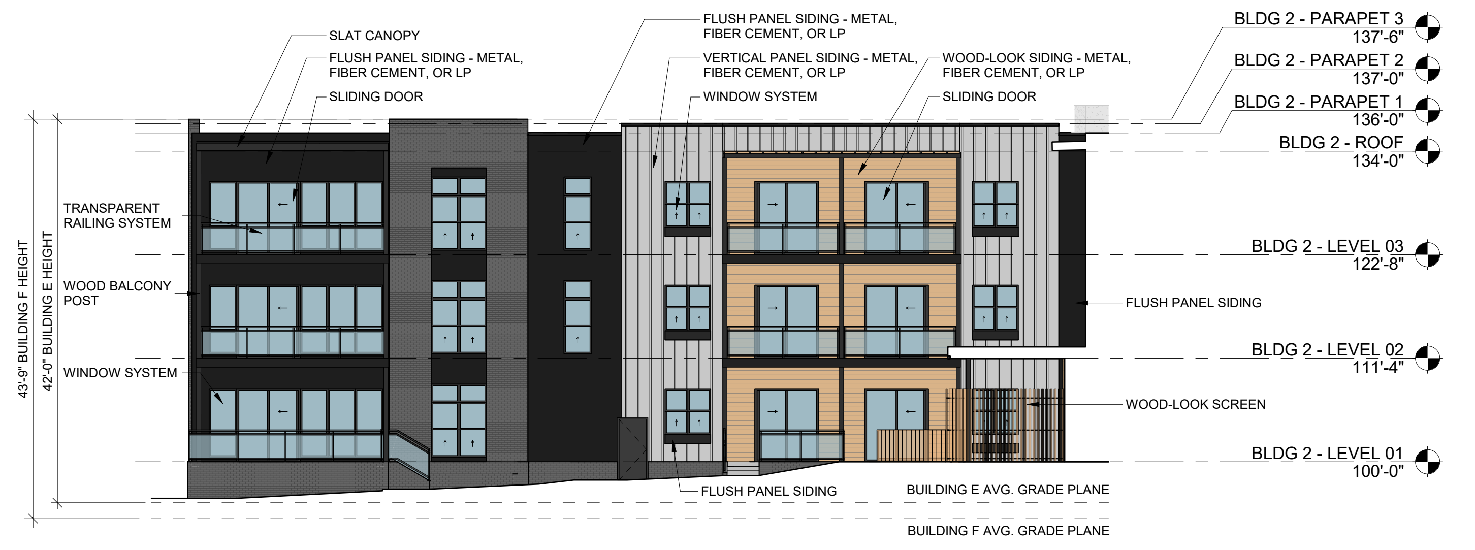
2 BUILDING E/F ELEVATION 3/32" = 1'-0"
