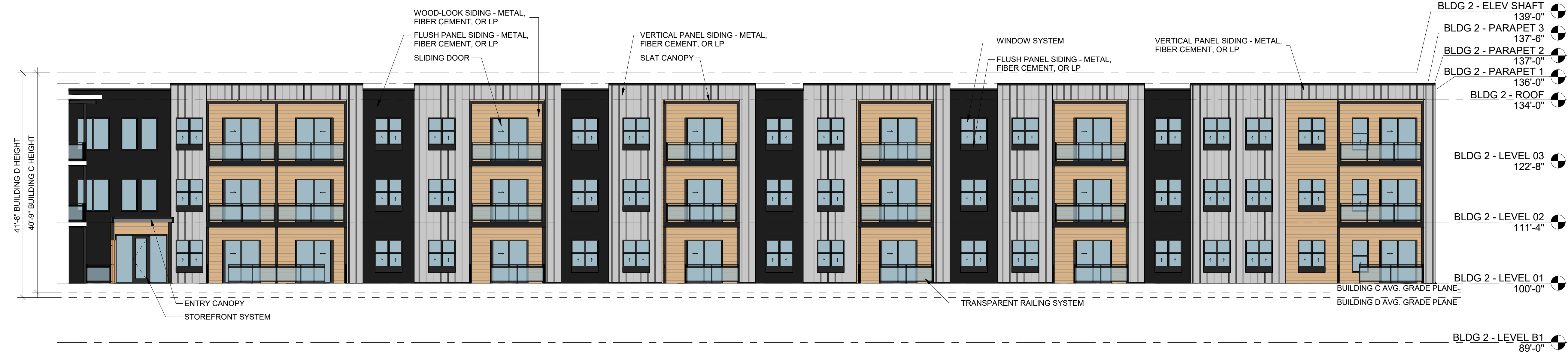
BUILDING C ELEVATION (BUILDING D 2 MIRRORED) 3/32" = 1'-0"
