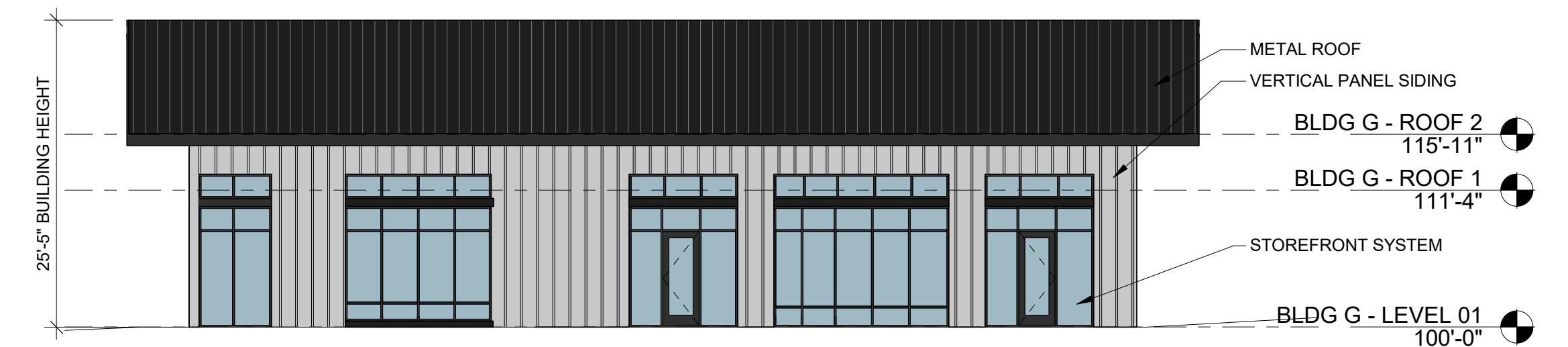
3 BUILDING G - NORTH ELEVATION 3/32" = 1'-0"
