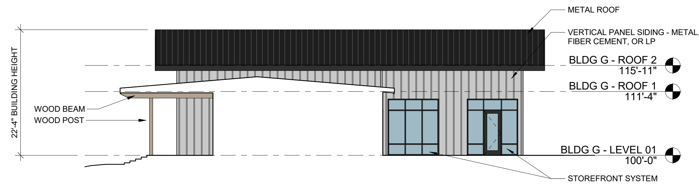
6 BUILDING G - NORTH ELEVATION 2 3/32" = 1'-0"
