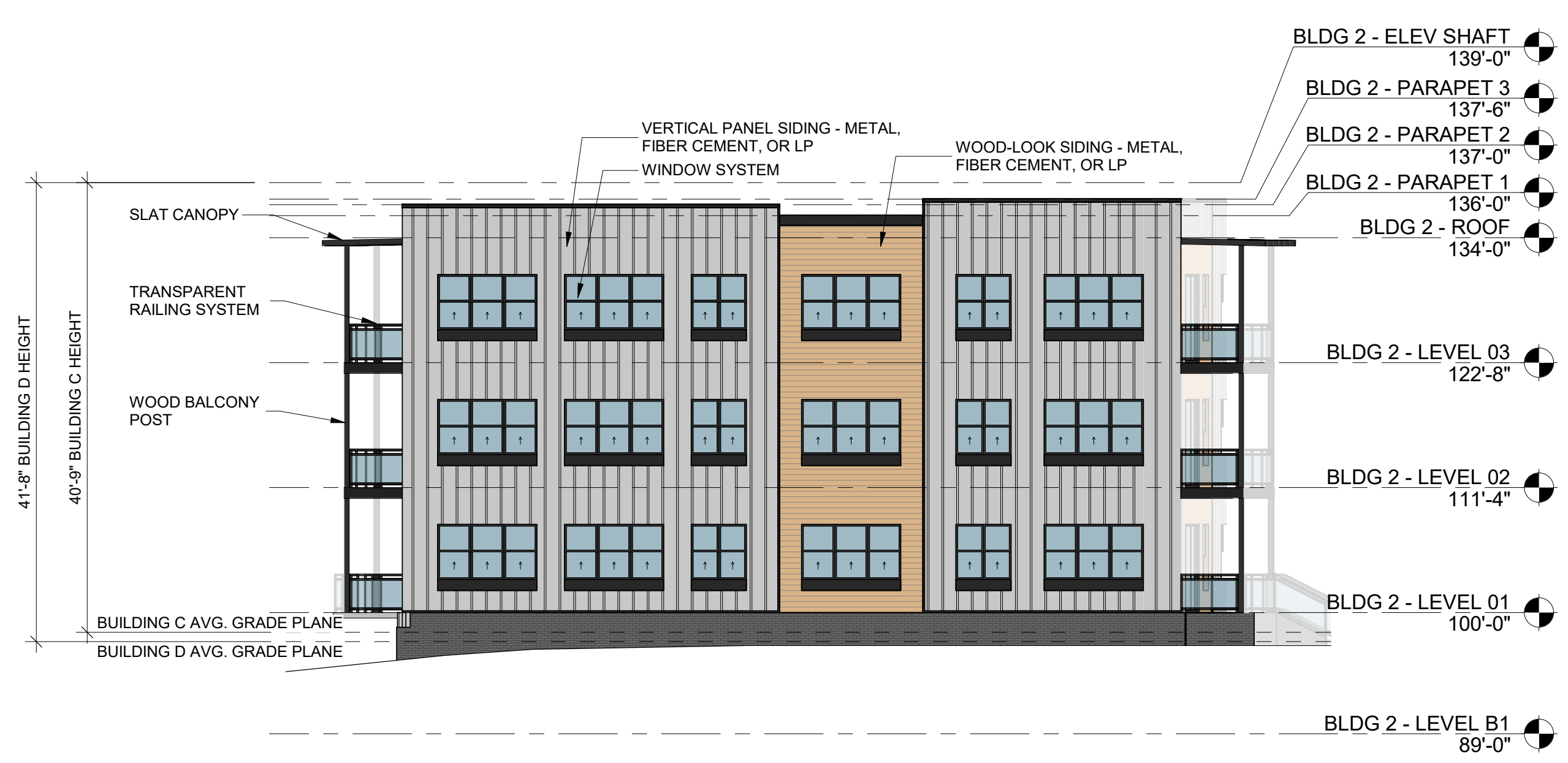
BUILDING C ELEVATION (BUILDING D MIRRORED) 6 3/32" = 1'-0"
