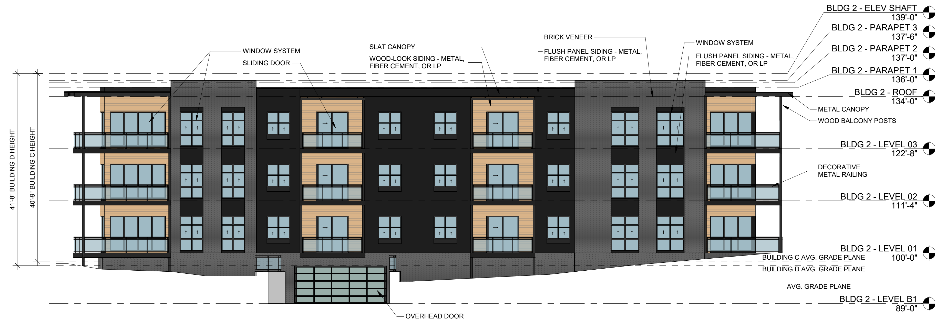
BUILDING C ELEVATION (BUILDING D 4 MIRRORED) 3/32" = 1'-0"
