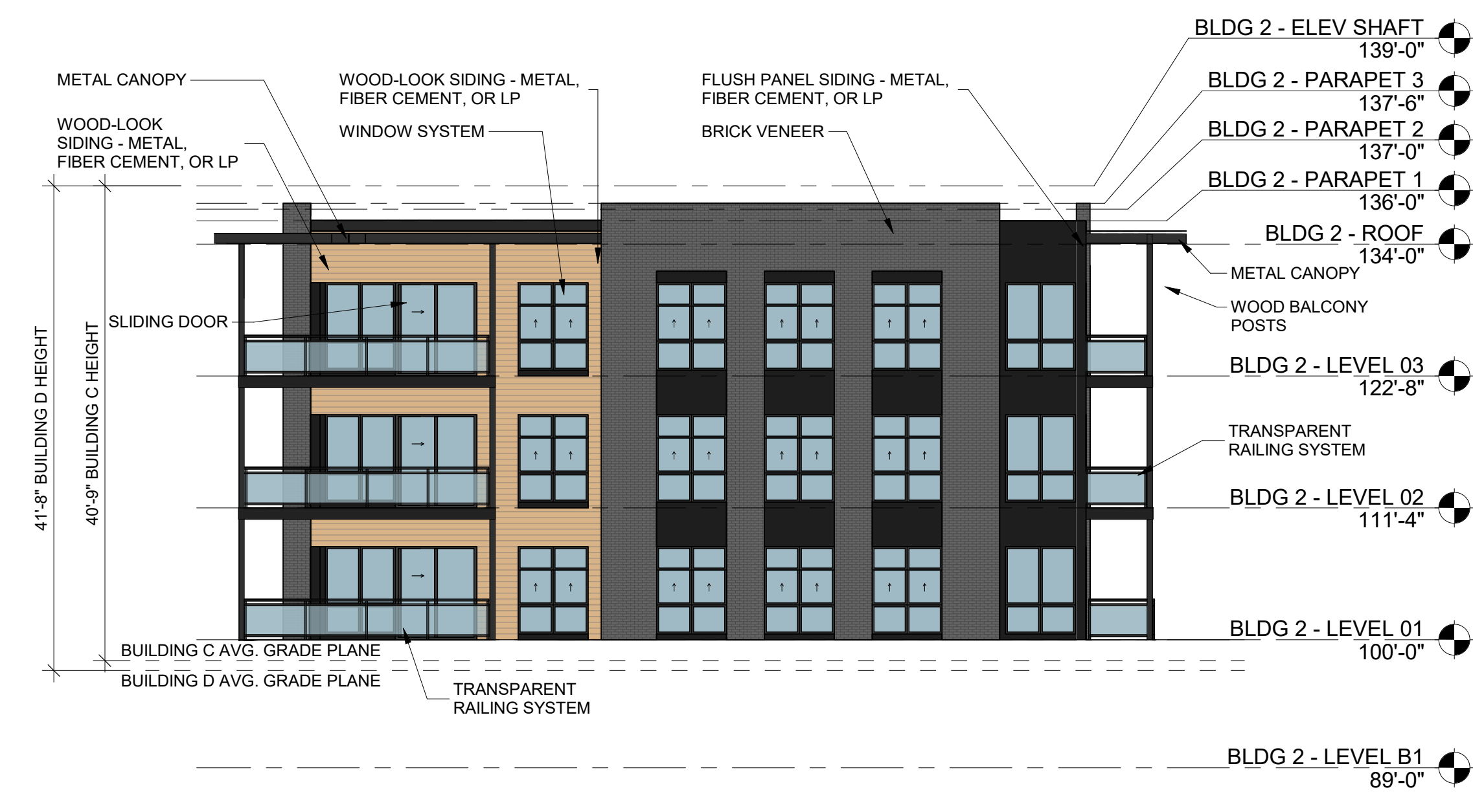
BUILDING C ELEVATION (BUILDING D 3 MIRRORED) 3/32" = 1'-0"
