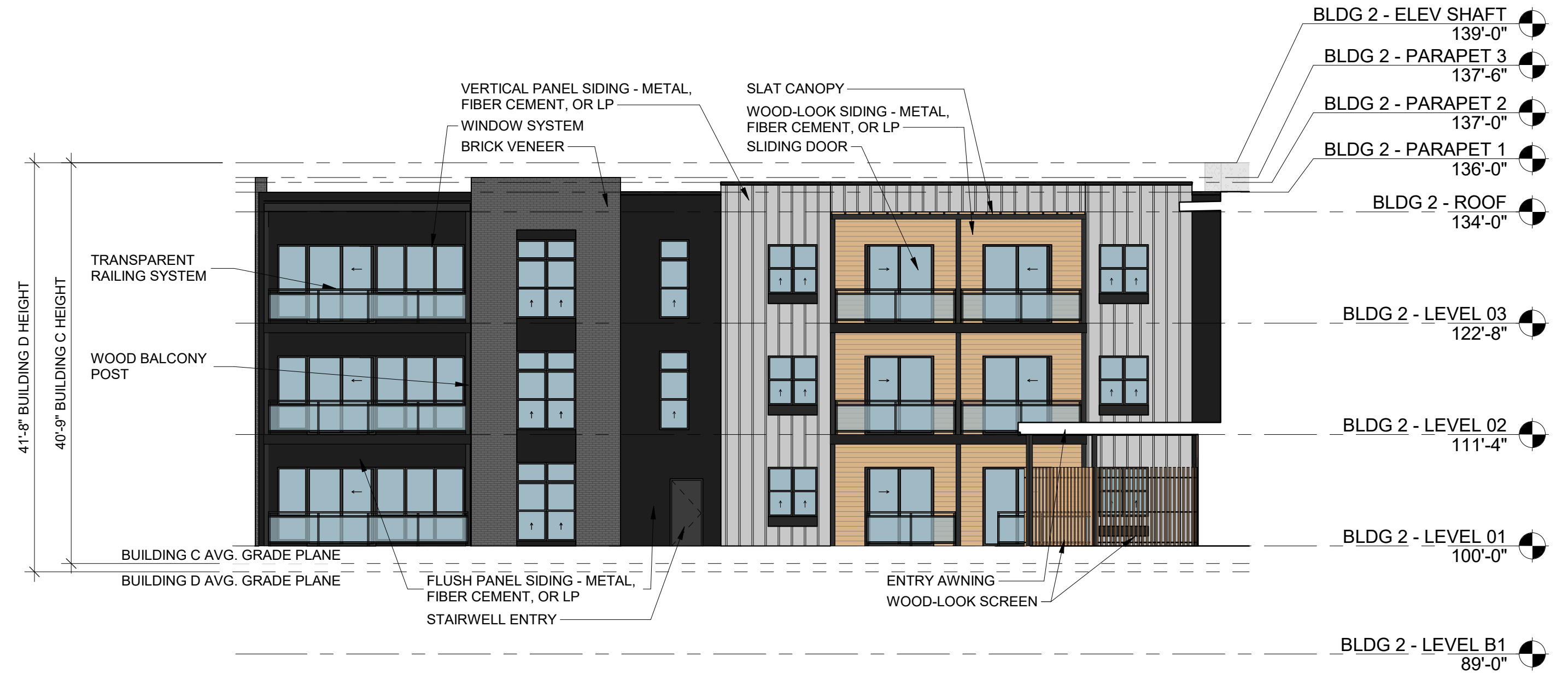
BUILDING C ELEVATION (BUILDING D MIRRORED) 5 3/32" = 1'-0"
