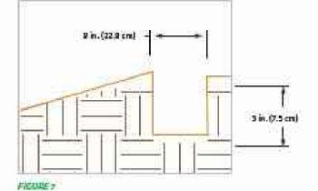
Place the wattle in the trench so that it contours to the soil surface. Compact soil from the excavated trench against the wattle on the uphil side. Wattles should
