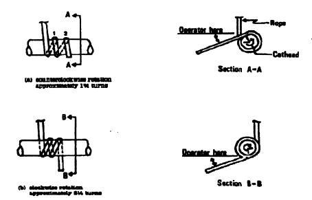
FIG. 1 Definitions of the number of rope turns and the angle for (a) counterclockwise rotation and (b) clockwise rotation of the cathead
