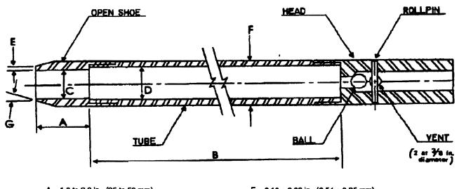
$E = 0.10 \pm 0.02 \text{ in. } (2.54 \pm 0.25 \text{ mm}) \\ F = 2.00 \pm 0.05 - 0.00 \text{ in. } (50.8 \pm 1.3 - 0.0 \text{ mm}) \\ G = 16.0^\circ \text{ to } 23.0^\circ$
