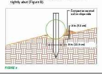
3. Secure the wattle with a minimum of 18 to 24 in. (45.7-61 cm) stakes every 3 to 4 ft (0.9-1.2 m) and with a stake on each end. Stakes should be driven through the middle of the wattle leaving at least 2 to 3 in. (5-7.5 cm). of stake extending above the wattle (Figure 9). Stakes should be driven perpendicular to the slope face. Spacing of SediMax-SW on slope will vary based on the slope grade (Figure 10).
