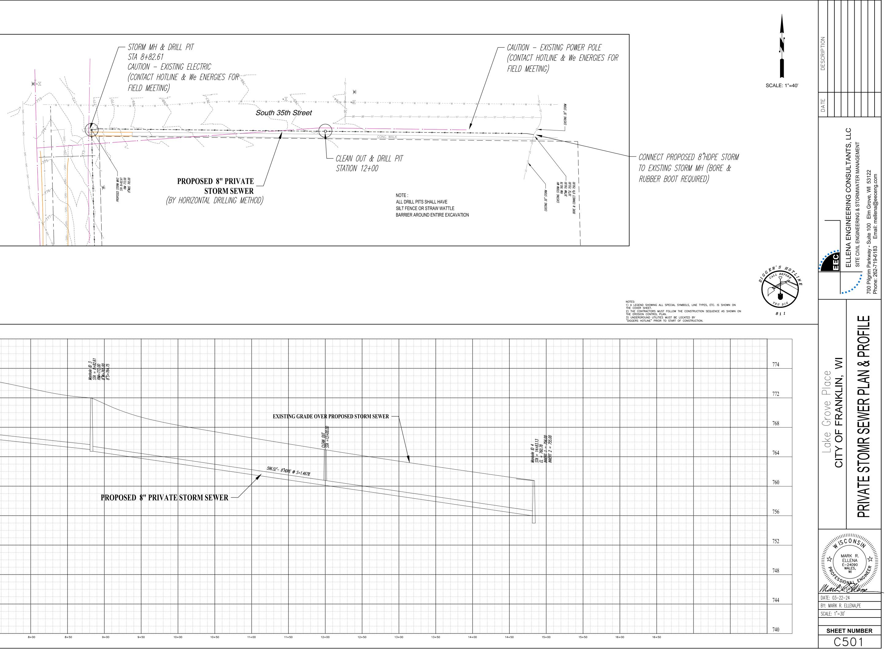
NOTE: ALL UNDERGROUND CONTRACTOR ARE REQUIRED TO FIELD LOCATE EXISTING UTILITIES, STORM SIZE & INVERT PRIOR TO CONSTRUCTION. OBTAIN ALL CITY PERMITS PRIOR TO CONSTRUCTION.
