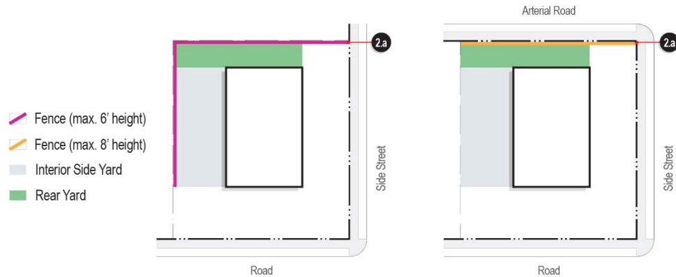
Figure 16 Fences on Lots with Single-Family and Duplex Uses in Interior Side and Rear Yards
